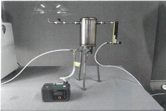
< Inlet(Mixing chamber at intake position)Sampling >
